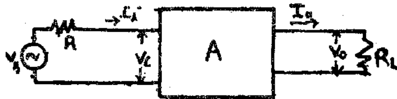
Fig. 6.4. Experimental set up to measure Amplifier parameters A = Amplifier; V_s = Signal source
