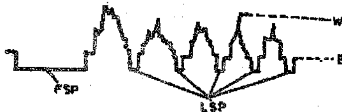
Fig 24.4 Composite Video signal FSP-Field Sync. Pulses LSP-Line Sync. Pulses W-White (picture brightness) B-Black (picture darkest)
