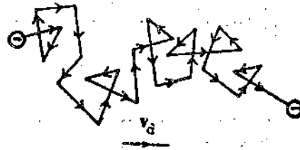
Fig 6.2 an impressed electric field causes the electrons to drift with a velocity V_d towards the right. What is the direction of E ?
