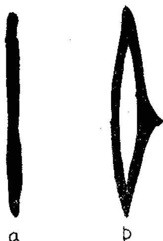
Fig.22.2 Traces obtained with Silver atoms, (a) Without field, (b) With field
